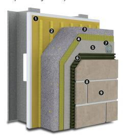
Substrate: Glass Mat Gypsum sheathing in compliance with ASTM C1177, Exterior or Exposure I wood-based sheathing (plywood or OSB), code compliant concrete, concrete masonry, or existing structurally sound, uncoated brick wall costruction
